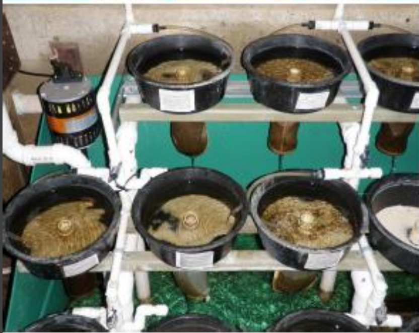
Top: Rearing pan system at Aquatic Wildlife Conservation Center, Marion, Virginia. Bottom: Close-up of the plastic culture pans, center drain, filter socks, and sump. Photo credit: Nathan Eckert, USFWS.
