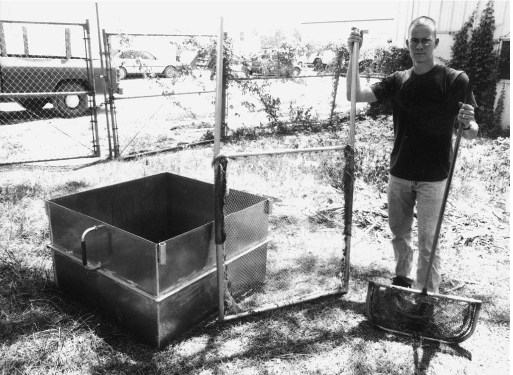
Figure 2. Equipment used to sample apple snails. From left to right; throw trap, bar seine, and dip net.
