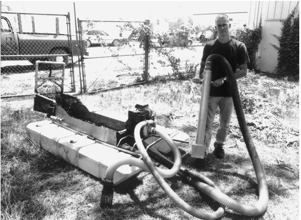
Figure 3. The suction dredge used to extract apple snails from throw traps. The pump, fluid transformer, and sorting tray float on the pontoons. Note that holes are needed in the bottom side walls of a throw trap extracted by a suction dredge to allow for water flow during the extraction process.
