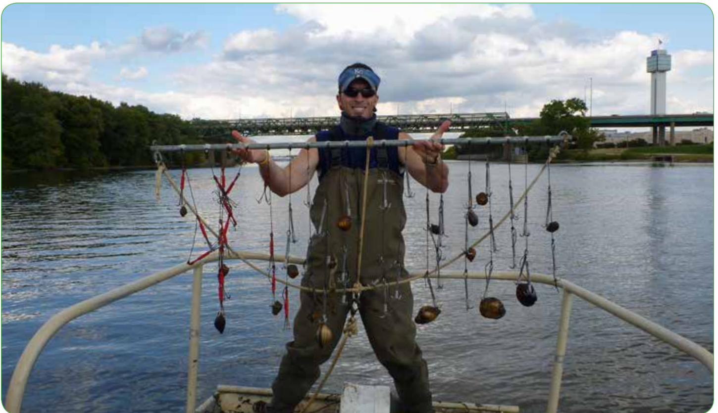
Figure 5 A brail (also called a crowfoot bar) with mussels attached to the hooks. Mississippi River, Illinois, USA.
